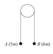
Two particles A and B have masses 5m and km respectively, where k < 5. The particles are connected by a light inextensible string which passes over a smooth light fixed pulley. The system is held at rest with the string taut, the hanging parts of the string vertical and with A and B at the same height above a horizontal plane, as shown in Figure 4. The system is released
