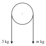
The particles have mass 3 kg and m kg, where m < 3. They are attached to the ends of a light inextensible string. The string passes over a smooth fixed pulley. The particles are held in position with the string taut and the hanging parts of the string vertical, as shown in the diagram above. The particles are then released from rest. The initial acceleration of each particle has magnitude  $\frac{3}{7}g$ . Find
