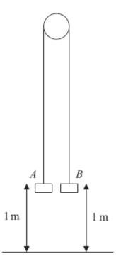
Two particles A and B have mass 0.4 kg and 0.3 kg respectively. The particles are attached to the ends of a light inextensible string. The string passes over a small smooth pulley which is fixed above a horizontal floor. Both particles are held, with the string taut, at a height of 1m above the floor, as shown in the diagram above. The particles are released from rest and in the subsequent motion B does not reach the pulley.
