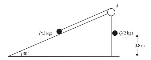
The diagram above shows two particles P and Q, of mass 3 kg and 2 kg respectively, connected by a light inextensible string. Initially P is held at rest on a fixed smooth plane inclined at  $30^{\circ}$  to the horizontal. The string passes over a small smooth light pulley A fixed at the top of the plane. The part of the string from P to A is parallel to a line of greatest slope of the plane. The particle Q hangs freely below A. The system is released from rest with the string taut.
